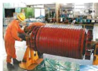
Inspection of high-voltage motor
